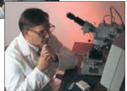
[After CAMS] Viewing automatically generated test results on a computer monitor linked to a microhardness tester with the CAMS upgrade.
